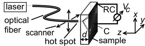
Fig. 1. Scheme of the experimental setup. A laser beam is coupled into an optical fibre, the end of which is brought close to the sample surface. An area with  $\sim 5\mu\text{m}$  in diameter is illuminated with some mW and carriers are excited thermoelectrically. To detect a pattern the fibre is scanned over the surface and the voltage  $V_C$  between the collector contact C and the reference contact RC on the sample edge is detected as a function of the fibre position.
