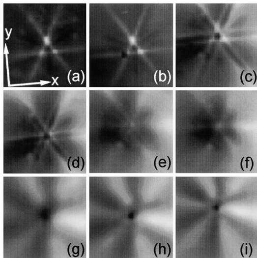
FIG. 2. Experimental focusing patterns for different values of the longitudinal magnetic field: The voltage  $V_c$  at the collector is shown in gray scale as a function of the fiber position. The image frame is approximately  $(450 \mu\text{m})^2$ . (a)  $B = 0$  T; (b)  $B = 1.1$  mT; (c)  $B = 1.7$  mT; (d)  $B = 2.3$  mT; (e)  $B = 2.8$  mT; (f)  $B = 4.5$  mT; (g)  $B = 25$  mT; (h)  $B = 50$  mT; (i)  $B = 75$  mT.
